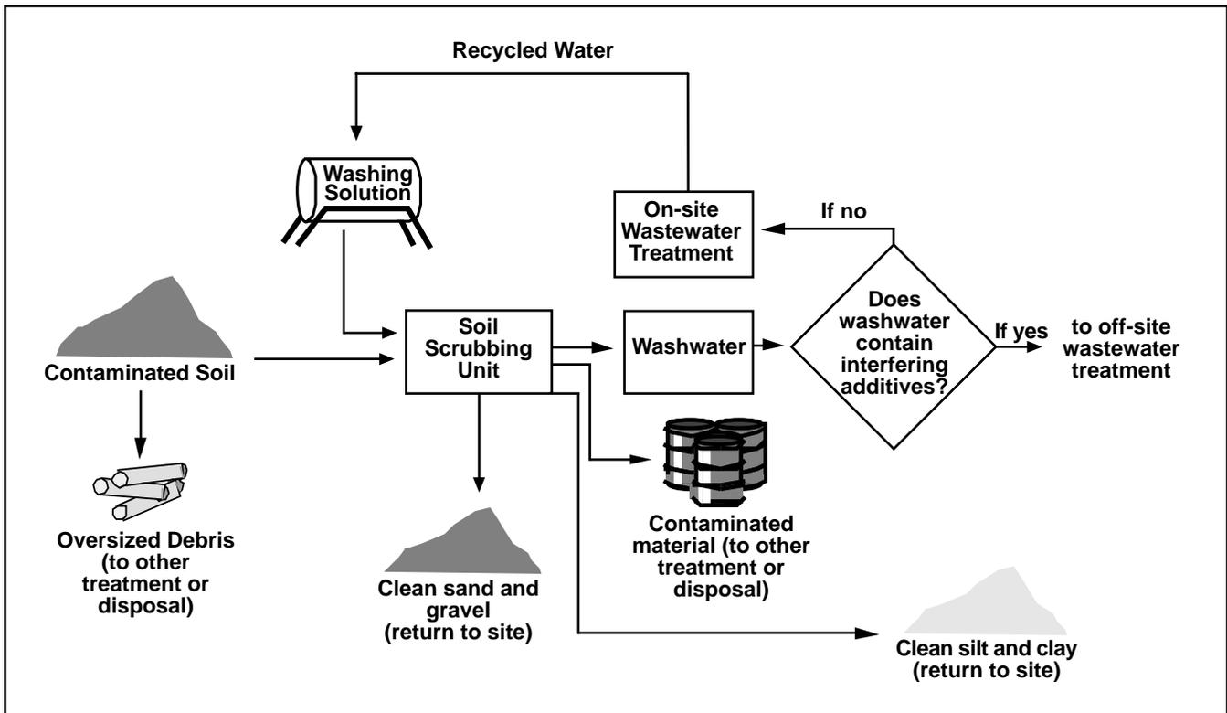
Ideally, the soil washing process would lead to a volume reduction of about 90% (which means only 10% of the original volume would require further treatment). Wastes with a high percentage of fine silt and clay will require a larger quantity of material to go on to subsequent, more expensive treatment. These soils may not be good candidates for soil washing.
